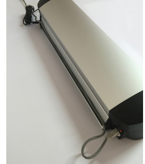
Guide the cable in the tray to avoid interfering with the measurement target.
